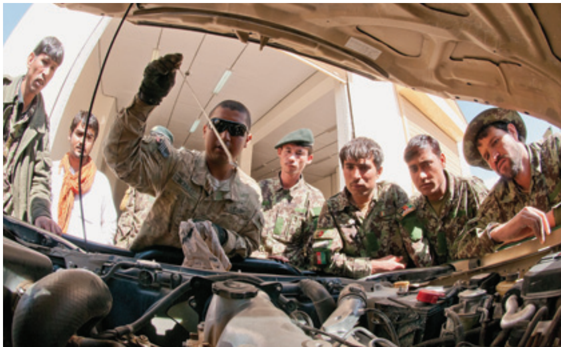
SPC Louis Morales, a mechanic with the 307th Brigade Support Battalion, explains to Afghan National Army drivers how to properly read a dipstick during preventive maintenance.
